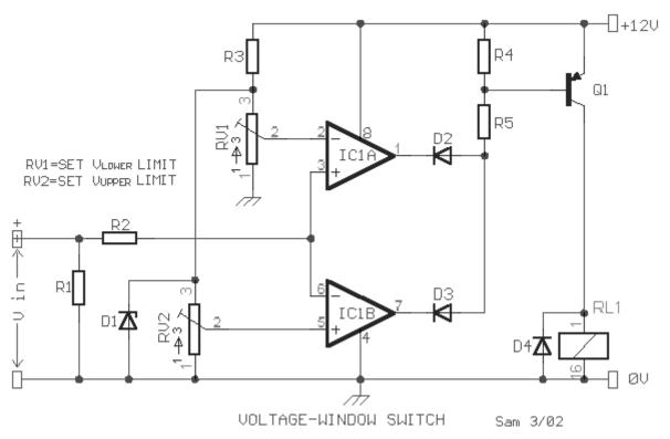
A voltage window switch is in practice the basic lower window limit of this circuit is roughly 3V and the upper limit is 9V. The window range can be extended by fitting a suitable range
