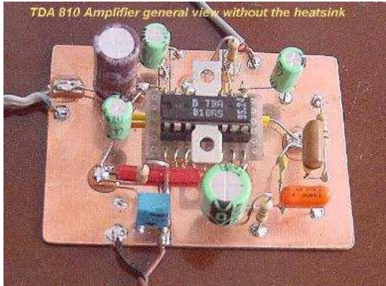
...built around the TBA 810 Integrated Circuit
