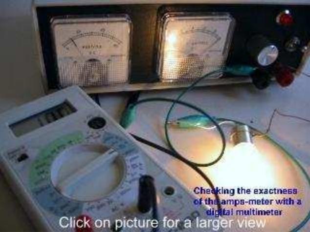
Now we proceed with the ampmeter. Again, we need a load resistor, which would be the 12 volt/15 watt bulb used in the previous test. Set the DVM in the amps' position and chose an appropriate range...for example, from zero to 10 amps, making sure it is always superior to 1.5
