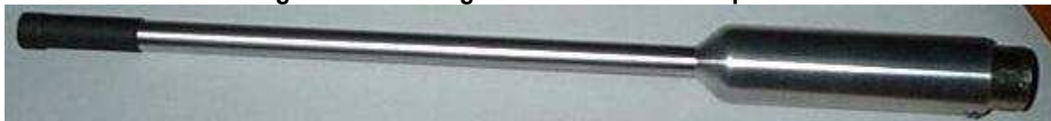
Figure 4b - My Prototype Measurement Mic Probe
