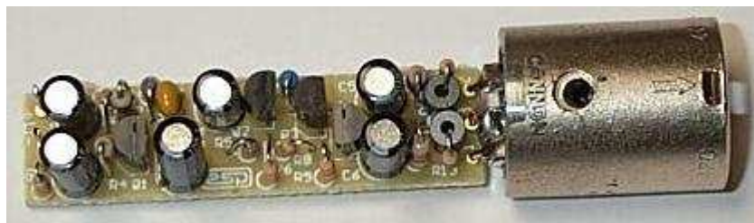
Figure 4c - Photo of Completed Preamp
