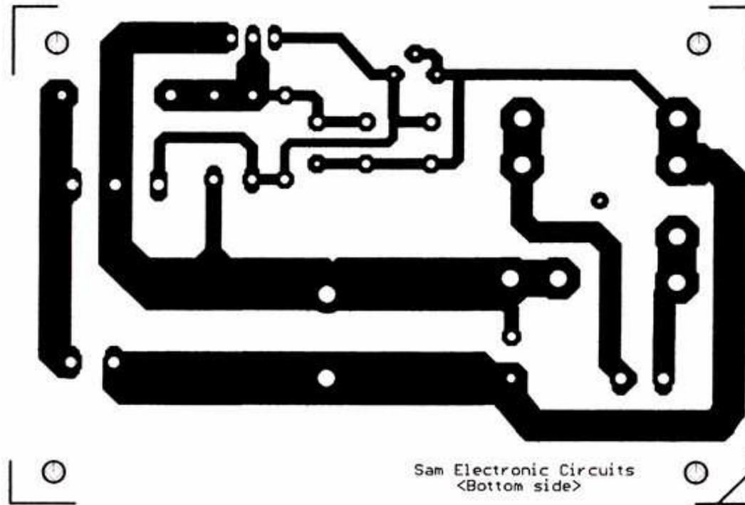
**Fig.3- Bottom side PCB.**
