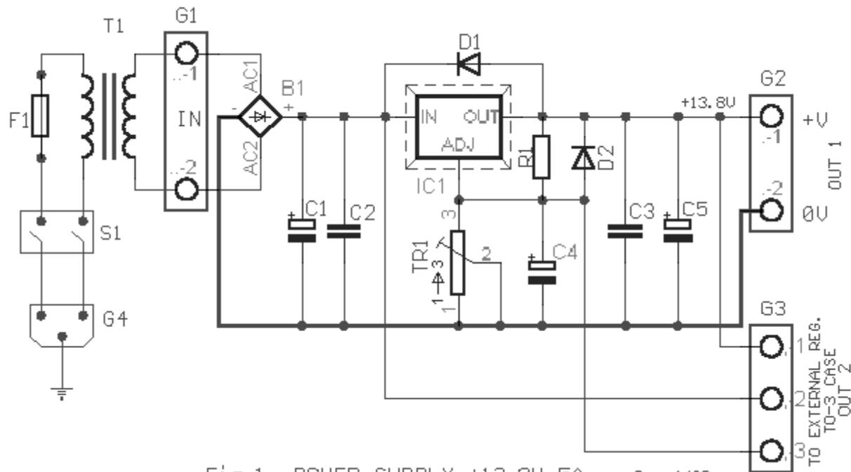
Fig.1- POWER SUPPLY +13.8V 5A Sam 4/02
