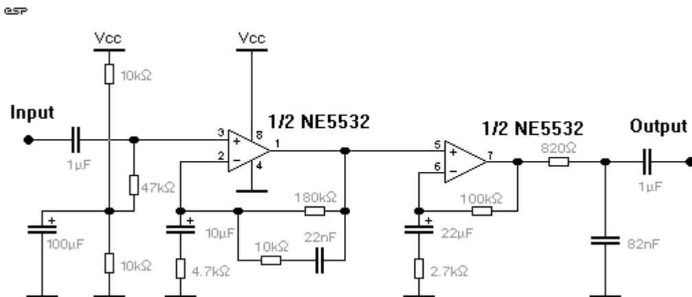
Figure 2 - Single Supply Version (Modified Pinouts)
