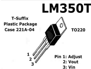
Heatsink surface connected to Pin 3.
