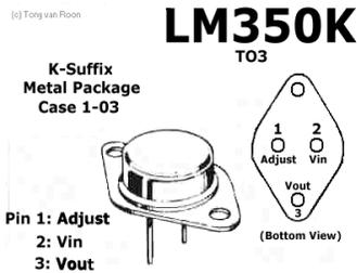
Pin 1 and 2 electrically isolated from case.
