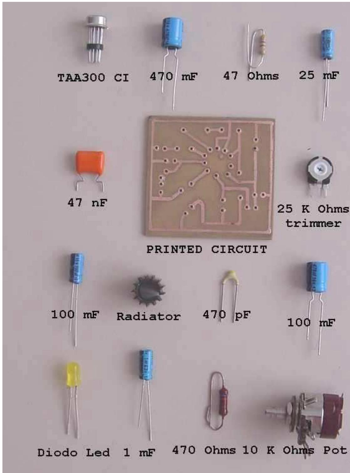
Other components that you can add would be a LED, with a 470 ohm resistor to control the ON/OFF state of the amplifier; a switch (SPST), and an 8 ohm
